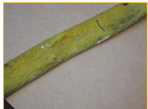
**Figure 4** Surface fibres damaged by abrasion
