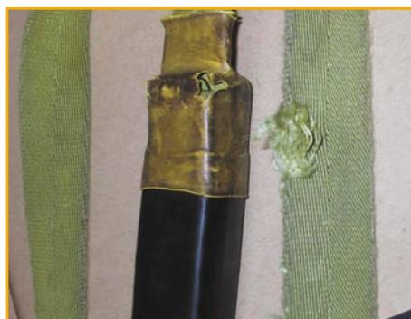
**Figure 1** Damaged webbing and protector to energy absorber
